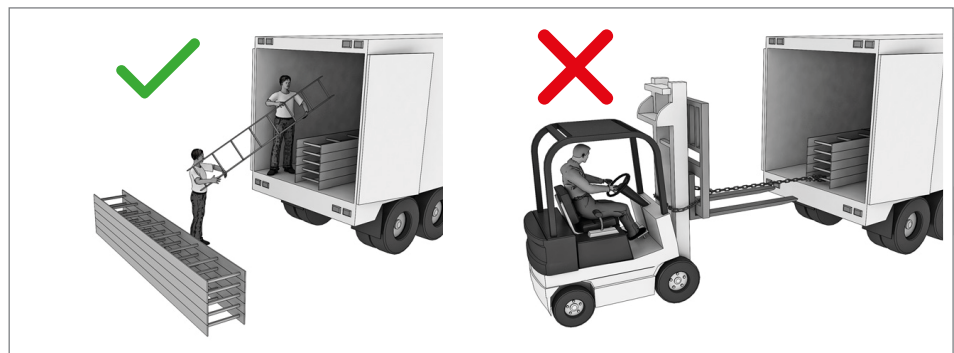
Fig. 1: Unloading the cable sections
